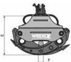
Example of Reinforced Forestry Grapple with application of Chainsaw Kit and Rigid Rotation
